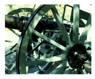
This unique Restoration Project was successfully completed by the skilled Joiners at Coleman & Fairburn. The work involved carefully stripping down the historic 1877 gun so that the metal components could be shot blasted and recoated in 2 pack protective paint.
